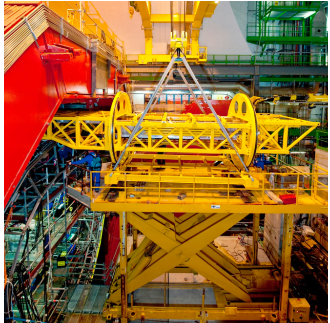
Figure 7.3: View of US-led ALICE ElectroMagnetic Calorimeter (EMCal) modules during installation in the ALICE experiment; one of the 10 EMCal modules, weighing over 7 tons, is being inserted.
